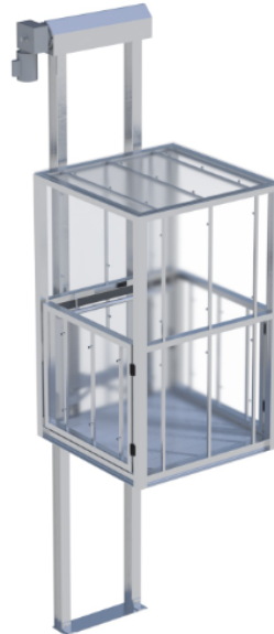
Figure 4: Specifications for proposed lift. I-beams will be sized to the height of the porch.
