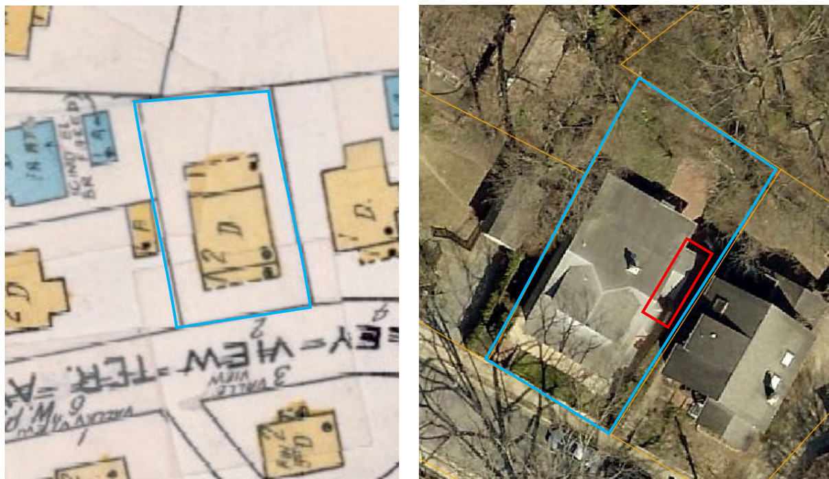
Figure 6: Sanborn fire insurance map (left; 1927-1963) and aerial photo (right; 2019) showing the subject property outlined in blue. The non-historic side addition with faux brick cladding is outlined in red.
