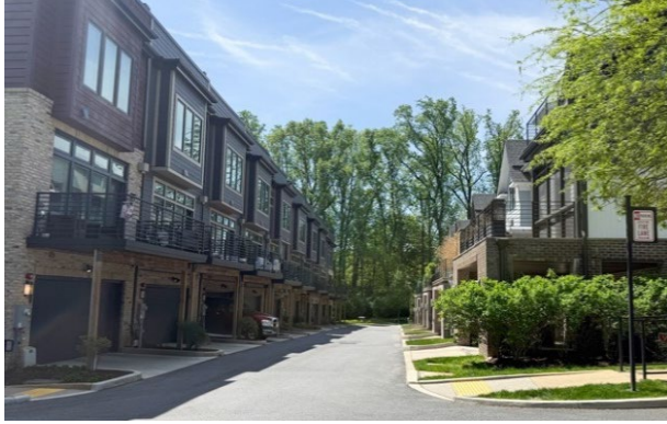
Figure 3. The perceived width of an alley is narrowed through several design elements: the pavement material changes between the driveways and alley, parking spaces are concealed by walls and dense landscaping along the street edge, and the building colors within the alley work harmoniously together.
