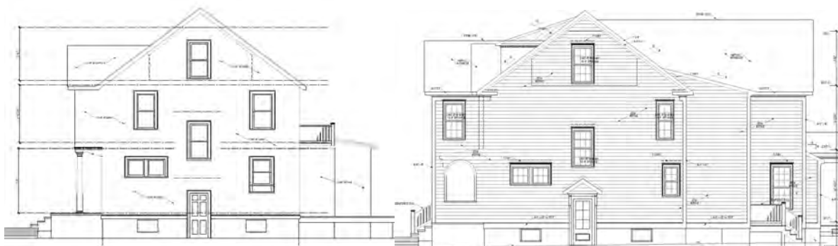
Figure 4: Existing west elevation (left) and proposed (right).
