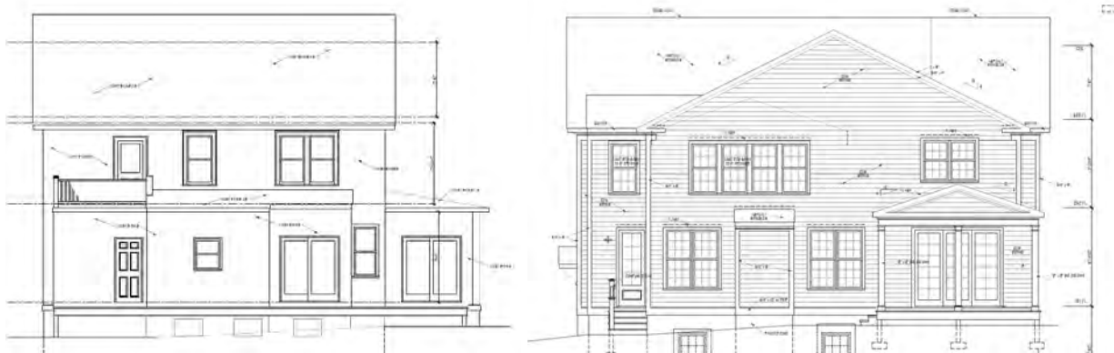
Figure 3: Existing rear addition (left) and proposed (right).
