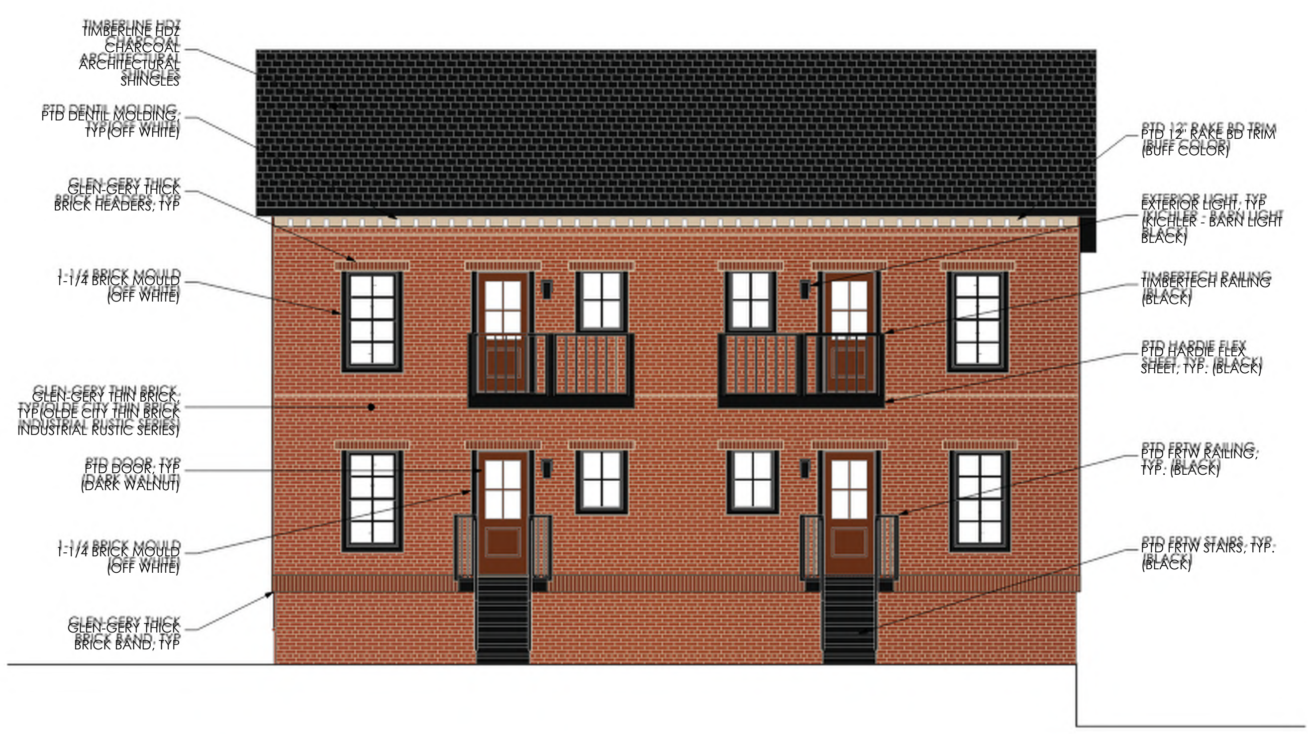
Front Elevation - Street View 3/16" = 1'-0"
