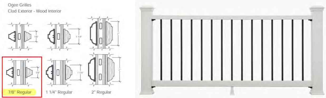
Figure 7: Proposed Pella simulated-divided-light, ogee grilles (left) and proposed Trex Select Classic porch railing (right).
