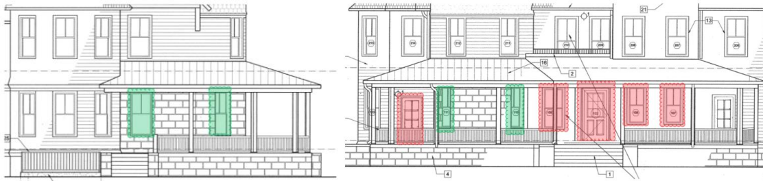
Figure 3: The three windows proposed for removal are located in the northeast corner of the house (shown in green).
