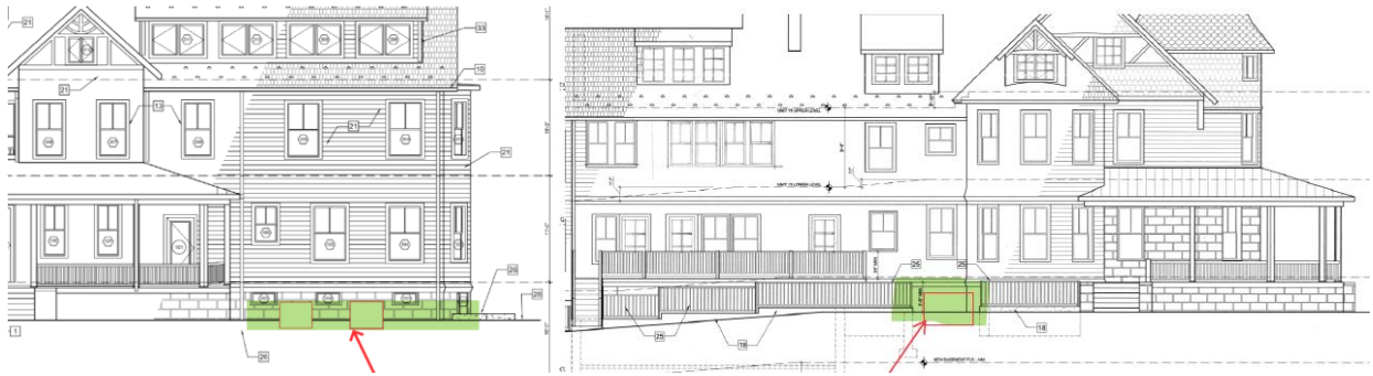
Figure 2: Two of the relocated HVAC units are on the north elevation (left) and one is on the east elevation (right).
