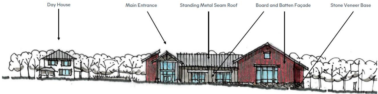
Figure 6: Site elevation along Stringtown Rd.
