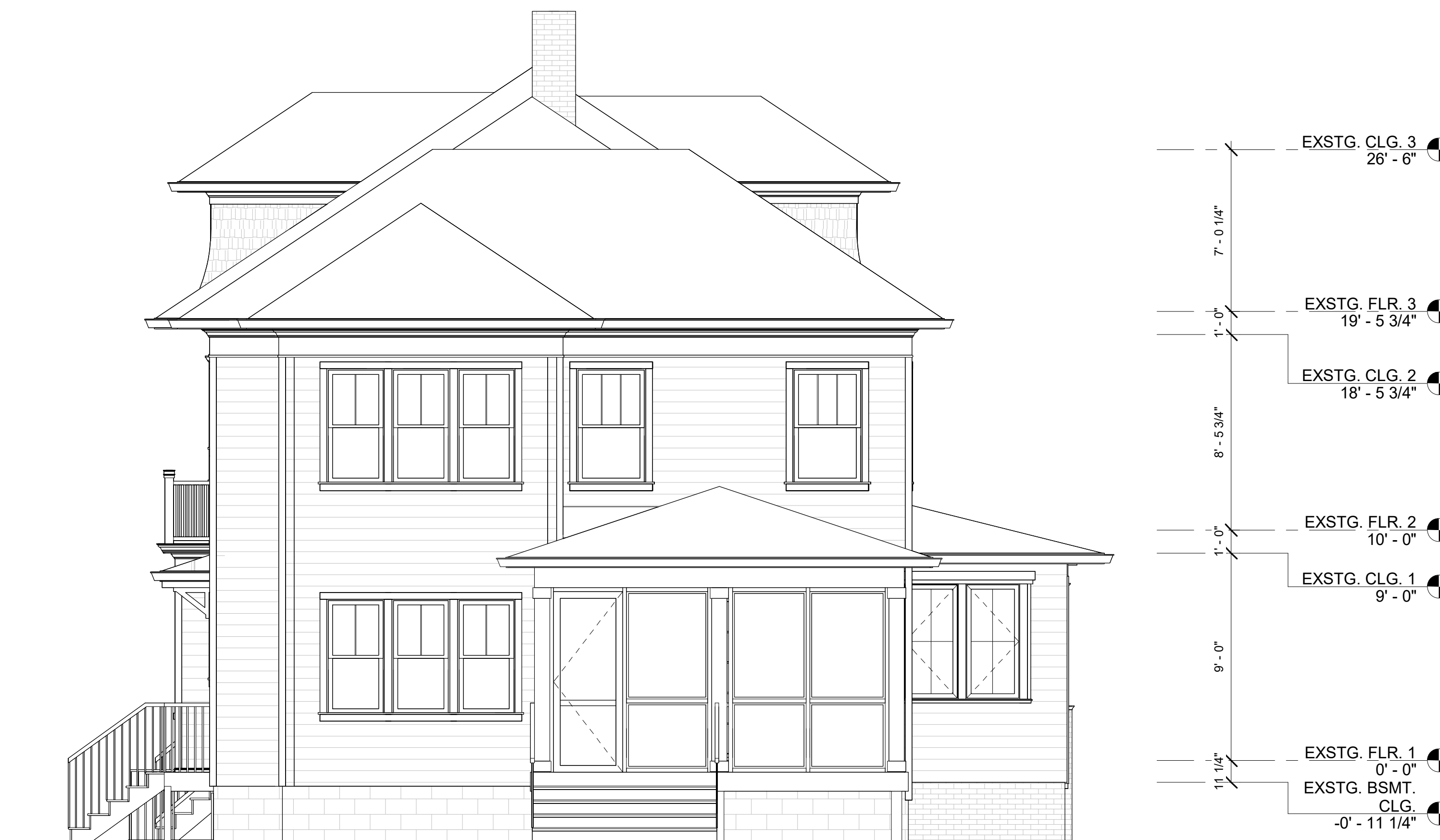
① Existing Rear Elevation 1/4" = 1'-0"
