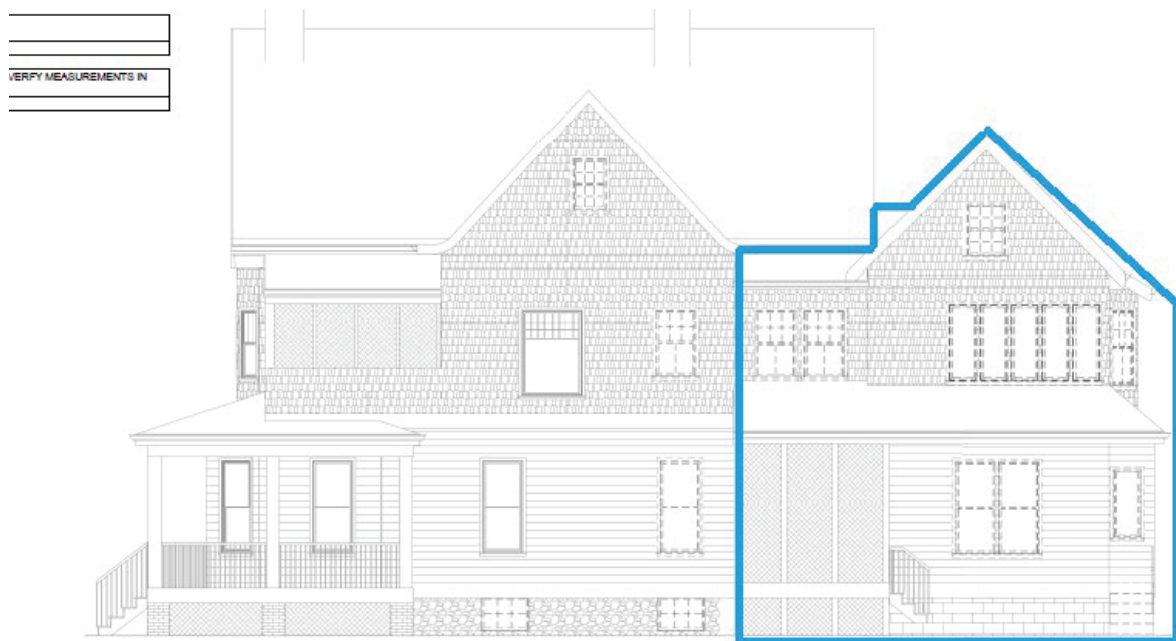
Figure 8: Existing west side elevation showing the windows proposed for removal/replacement. The non-historic rear addition is outlined in blue.
