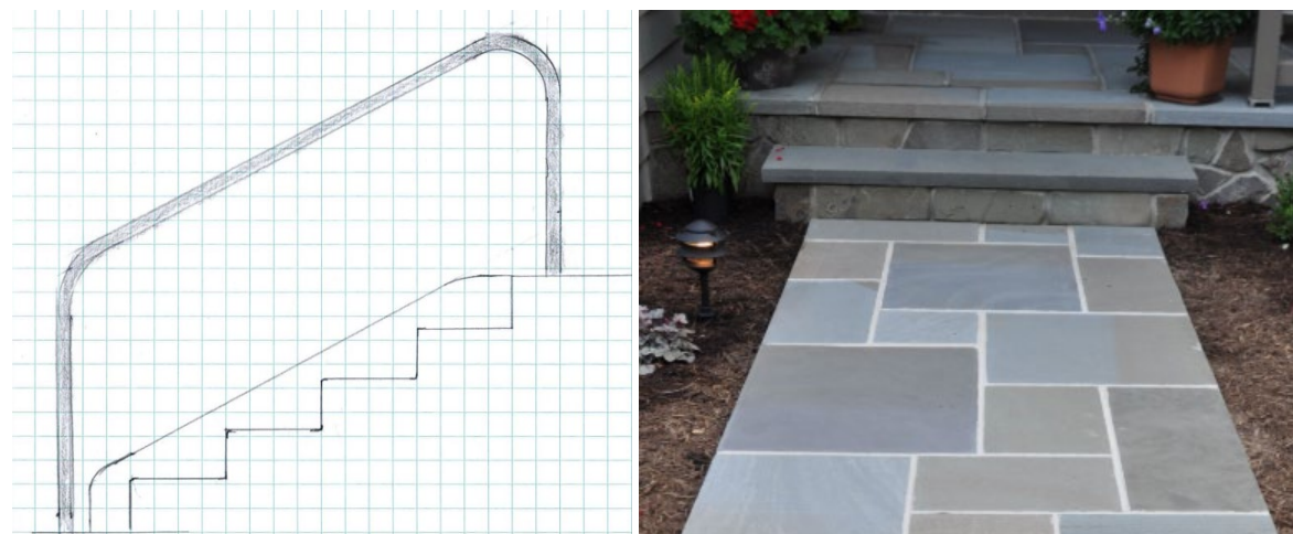
Figure 4: Proposed handrail between the sidewalk and front walkway, left; and proposed bluestone walkway and step material, right.
