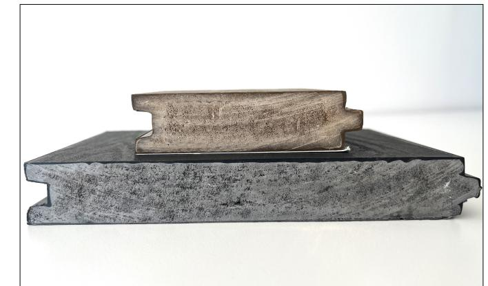
*Caption: PVC and composite decking can be produced with a tongue-and-groove profile.*
