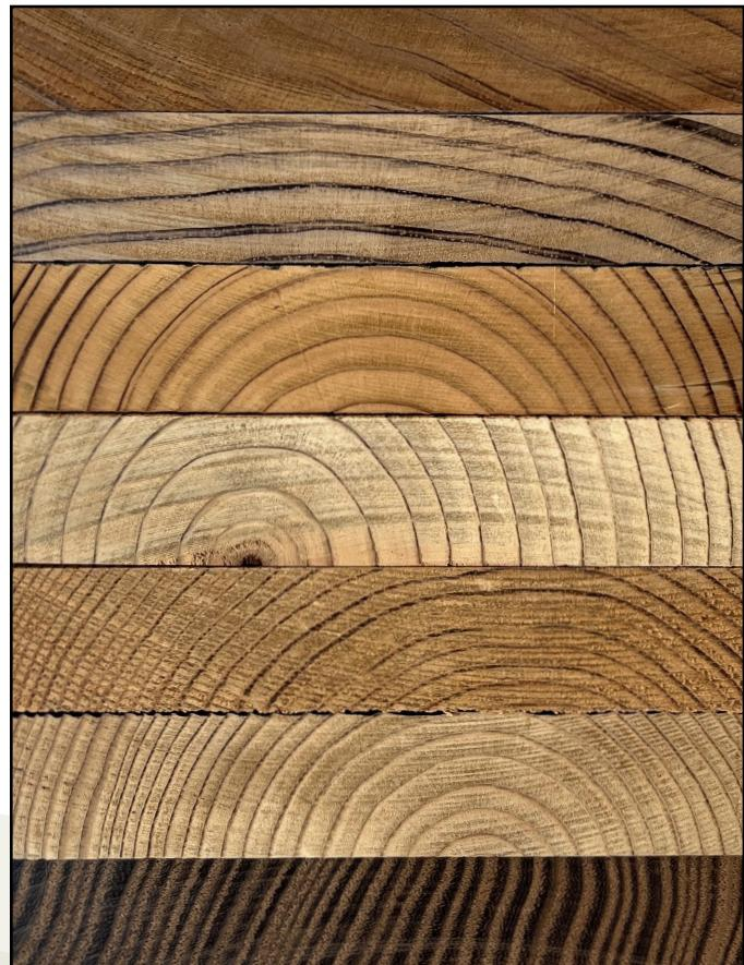
*Caption: The appearance and installation of this thermally treated wood is visually indistinguishable from stained lumber. Thermally modified Radiata Pine, Spruce, Scots Pine, and Ash.*
