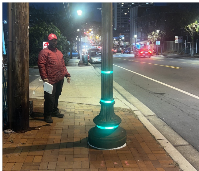
Reflective tape helps drivers see light poles.
