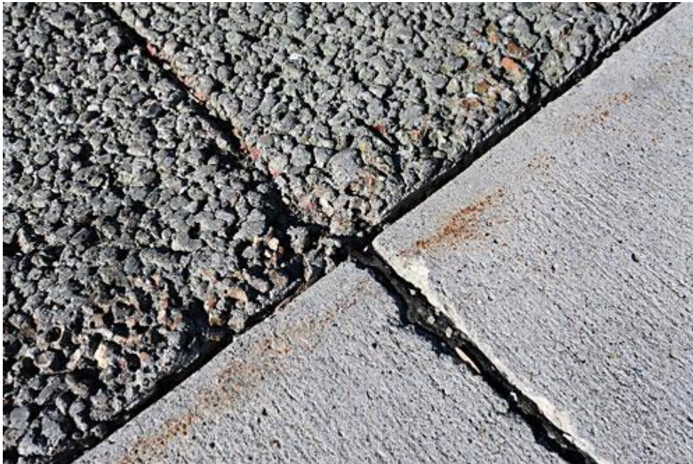
Figure 4: An example of permeable concrete (above) compared to contemporary concrete.
