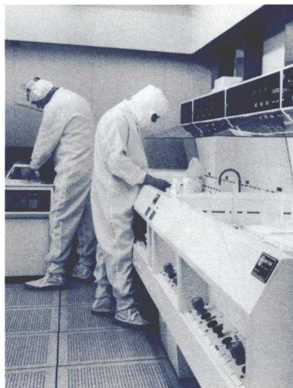
Figure 1. Class-100 clean room permits fabrication of MMICs with submicron geometry.
