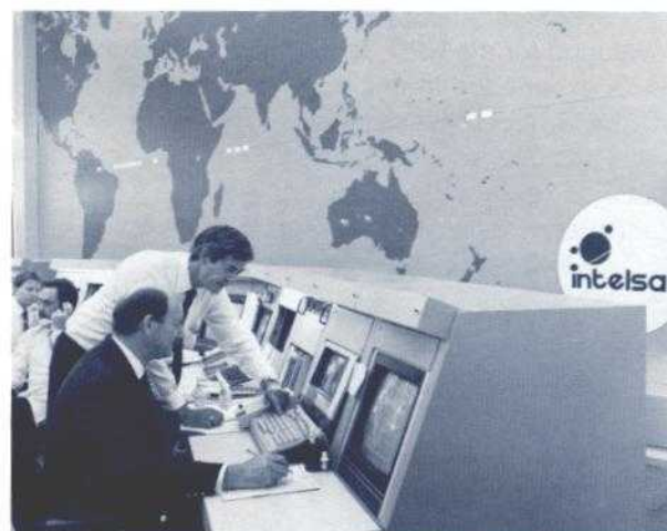
Figure 3. The INTELSAT Operations Center TDMA Facility provides centralized monitoring and control of TDMA satellite communications networks
