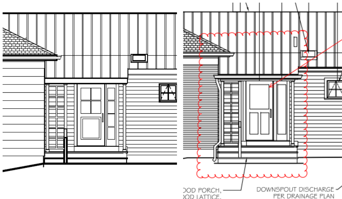
Figure 2: Approved design (left) and proposed revision (right).
