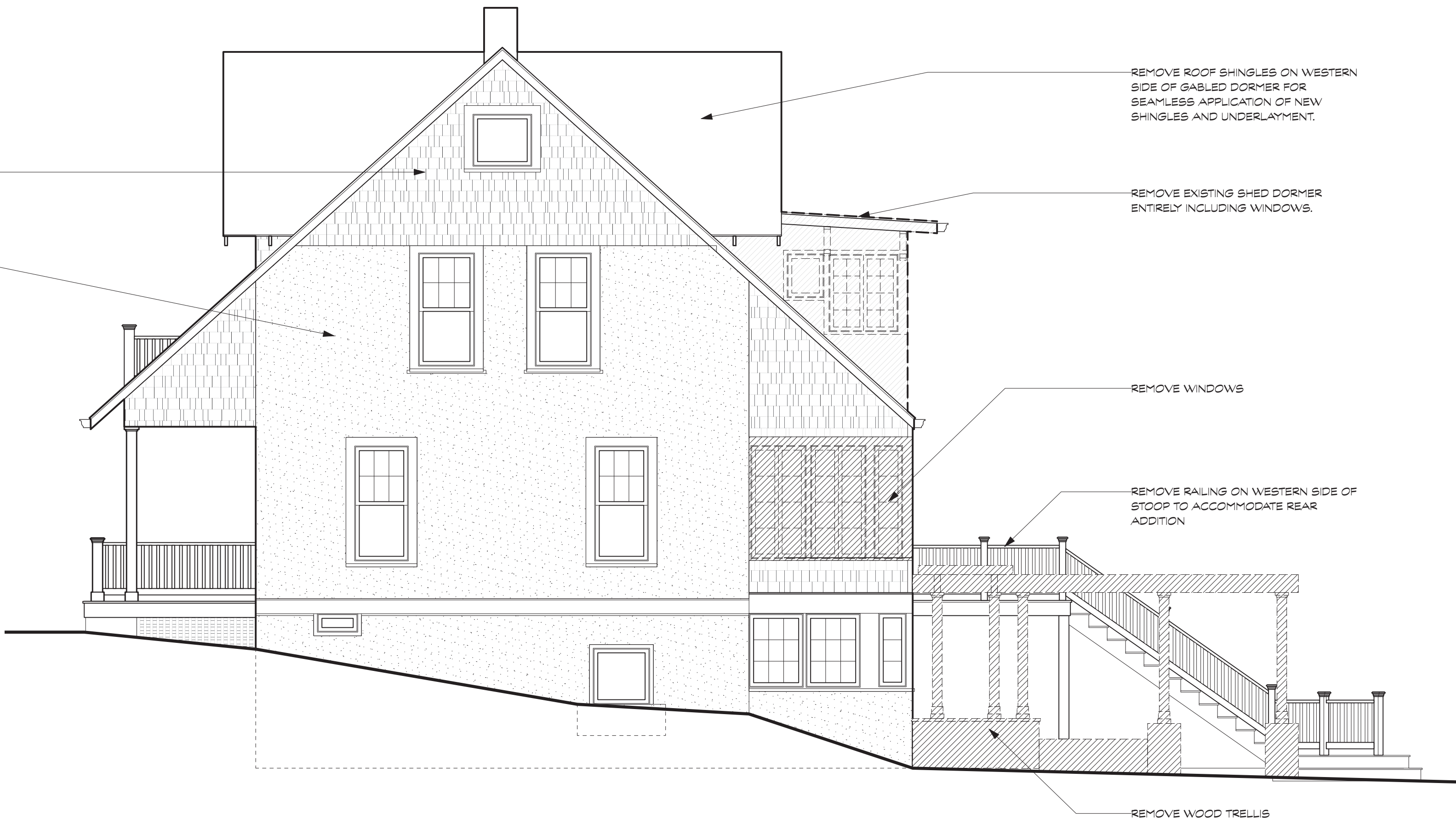
2 SIDE (WEST) DEMOLITION ELEVATION Scale: 1/4" = 1'-0"
