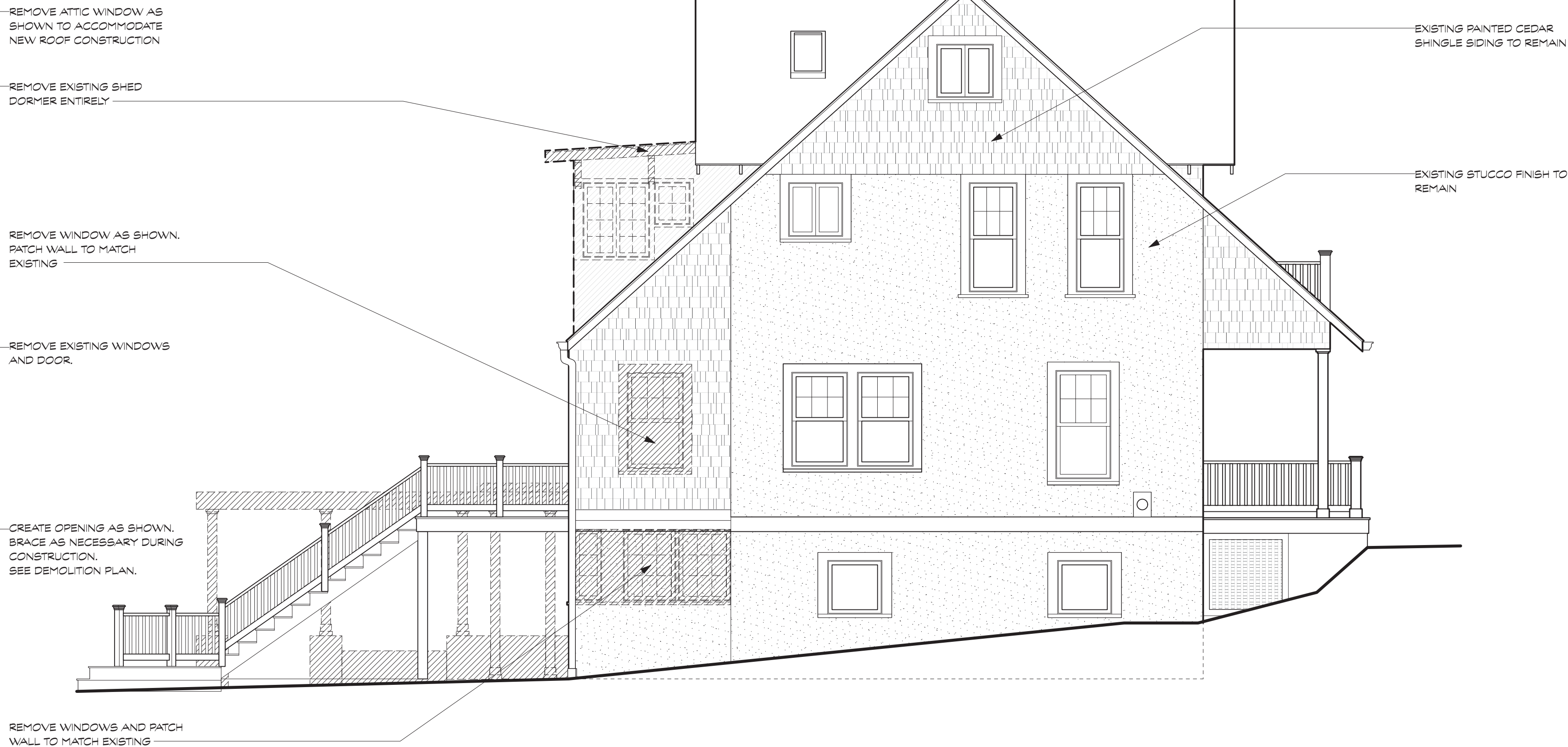
4 SIDE (EAST) DEMOLITION ELEVATION Scale: 1/4" = 1'-0"
