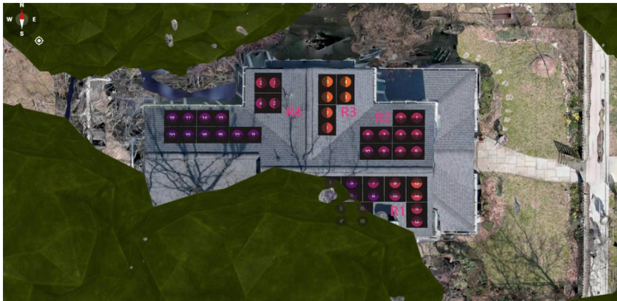
Figure 3: Roof heat map showing areas of highest solar collection.
