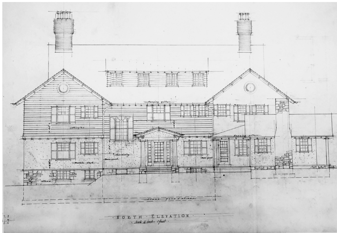
Architectural drawing of north elevation of John Joy Edson's country house by Arthur B. Heaton, showing original one-story kitchen wing on the right (demolished 1930) and modified front entrance (source: Arthur B. Heaton Collection, Library of Congress, Prints and Photographs Division)
