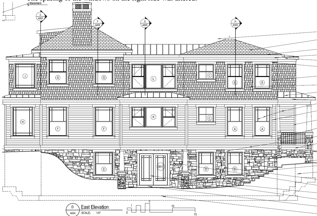
Figure 8: East Elevation (approved design).
