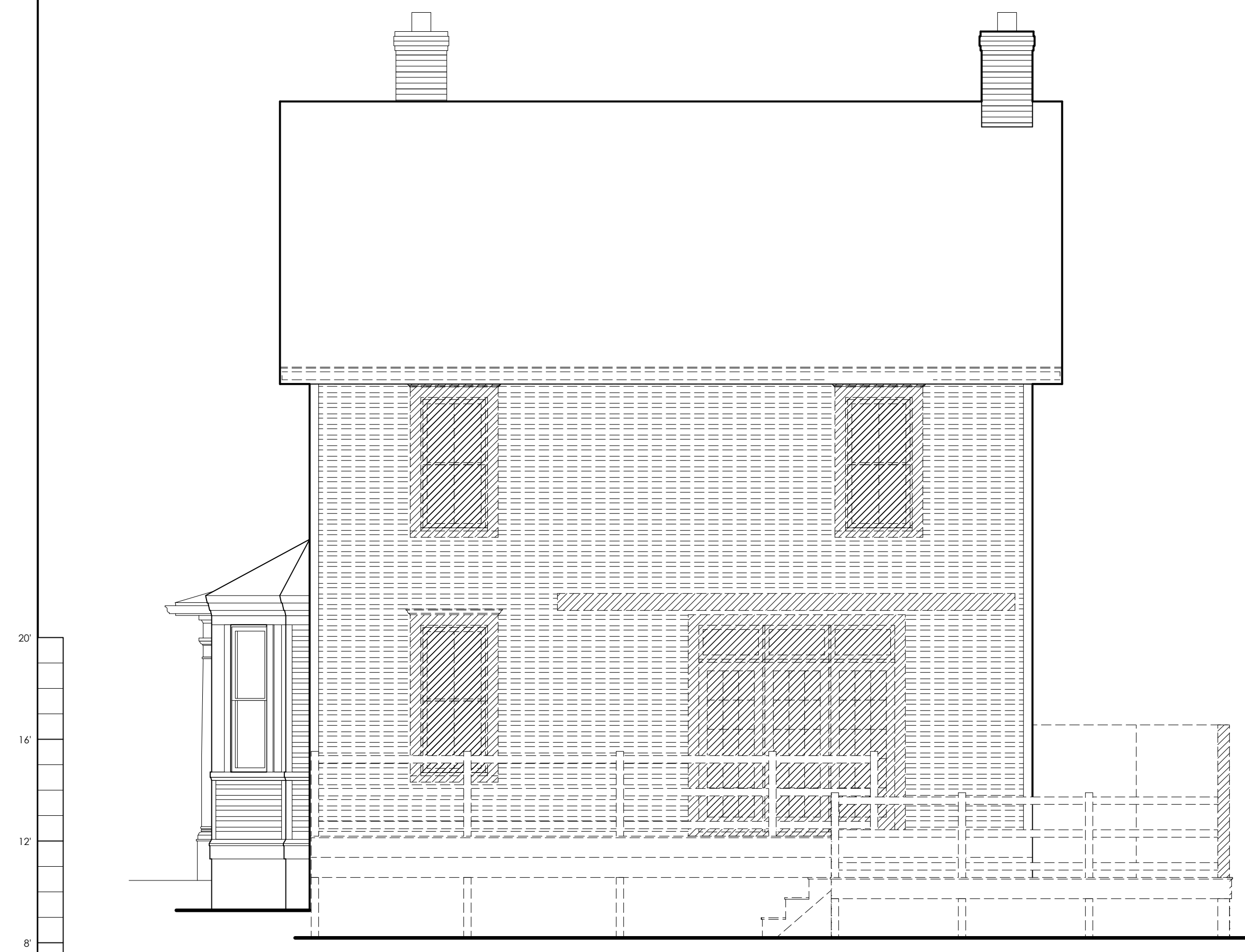
3 REAR DEMOLITION ELEVATION Scale: 1/4" = 1'-0"
