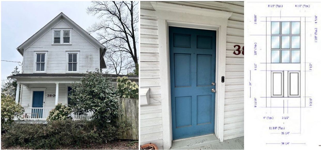
Figure 18: The existing (left and center) and proposed (right) front door of the historic house.
