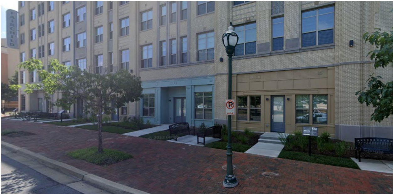
Figure 9. The ground floor of the Fairchild Apartments building was designed so that it would be possible in the future to convert the units to retail spaces. Image source: Google maps.
