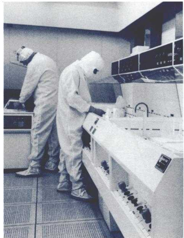
Figure 1. Class-100 clean room permits fabrication of MMICs with submicron geometry.
