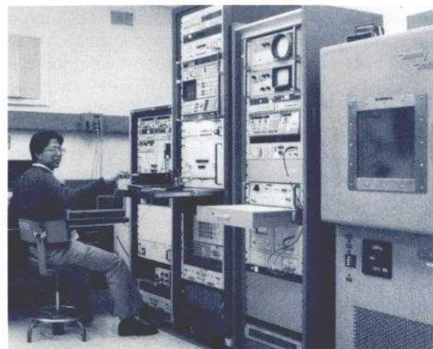
Figure 22. COMSAT Laboratories AMPAC system used for characterization of microwave power amplifiers and measurement control software
