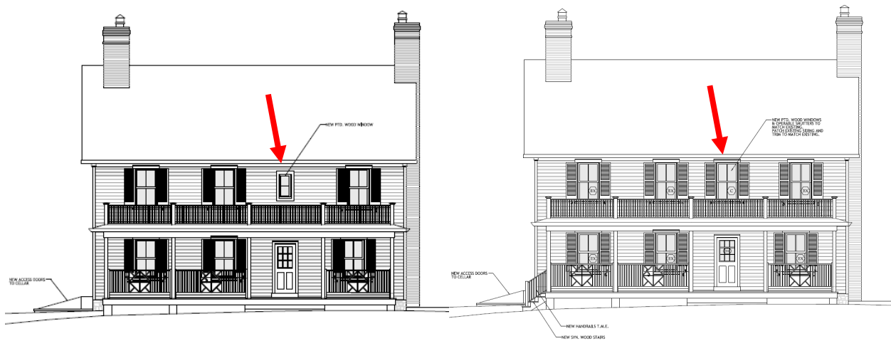
Figure 4: East elevation drawings, preliminary consultation proposal (left) and current proposal (right). The red arrow points to the location of the proposed window.
