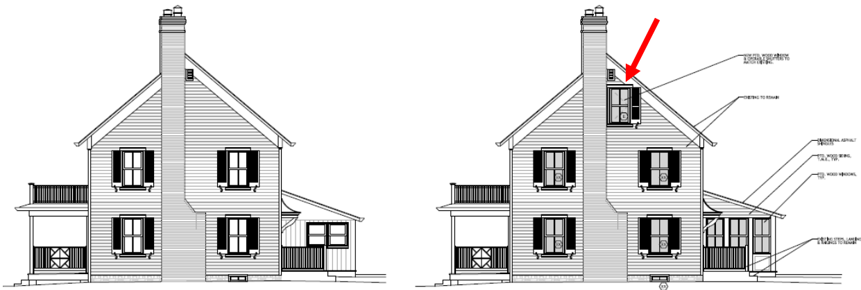
Figure 13: North elevation drawings, existing (left) and proposed (right). The red arrow points to the proposed casement window.
