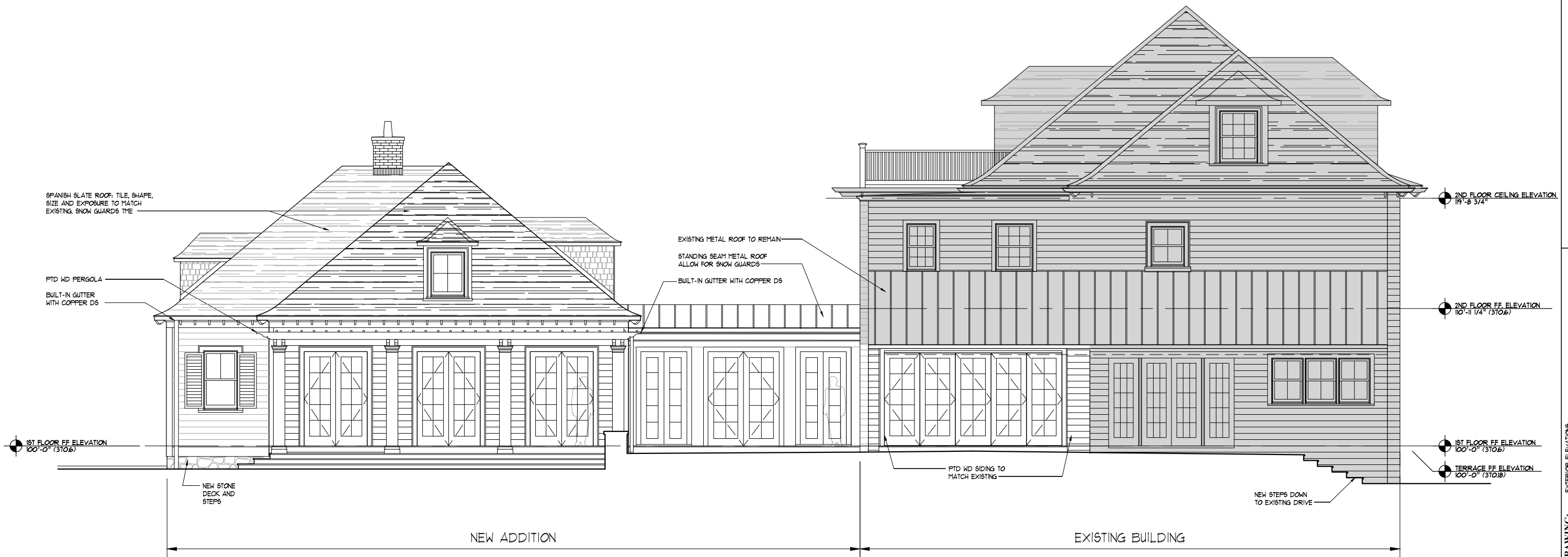
C1 BUILDING ELEVATION - SOUTH A4-3 1/4" = 1'-0" WHEN PRINTED AT 22"x36" 1/8" = 1'-0" WHEN PRINTED AT 11"x17"
