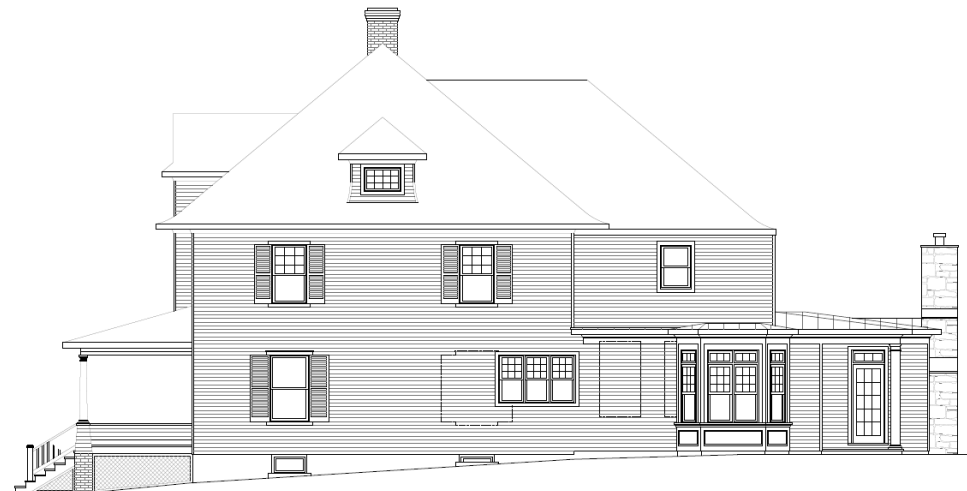
Figure 14: The proposed west elevation removes a historic first-floor window and replaces it with three smaller windows in a new opening that spans the end of the original rear wall.
