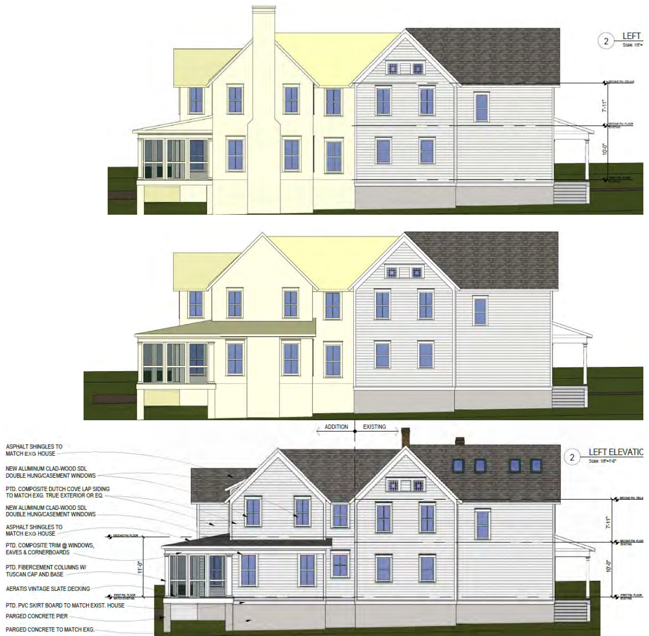
Figure 5: East (left) elevation as proposed in the preliminary consultation (top), during the preliminary consultation review (middle), and the current proposal (below).
