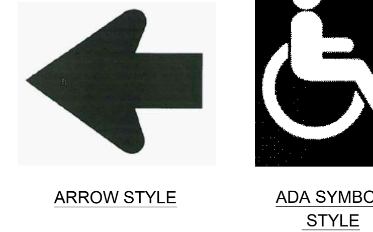
4 ADA DIRECTIONAL SIGN DETAILS NOTE: SIGN PANEL SIZE AND GRAPHICS UNDER DEVELOPMENT. PANEL SIZE WILL NOT EXCEED 12" x 12". SCALE: 1"=1'-0" 0 6" 1' 2' Scale: 1" = 1'-0"
