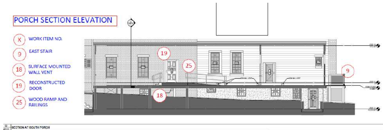
Figure 16: Porch section elevation.
