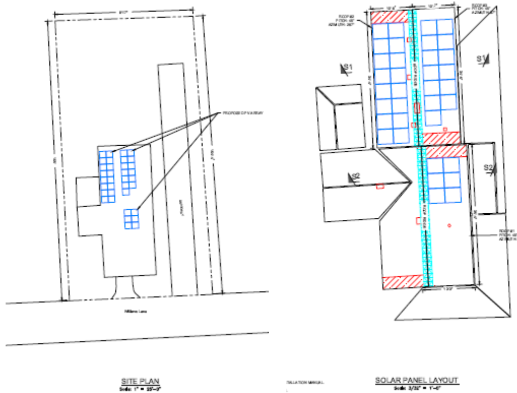
Figure 3: The site plan (left) shows the proposed solar panel locations and the building’s orientation toward Williams Lane. The roof plan (right) shows the proposed location of the solar panels.
