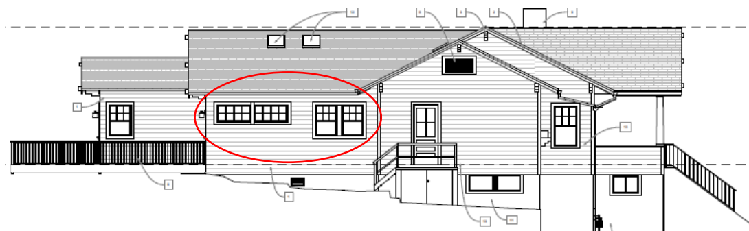
Figure 13: The proposed south elevation. New, compatible fenestration would be added to the existing wall of the non-historic addition being incorporated into the new addition.
