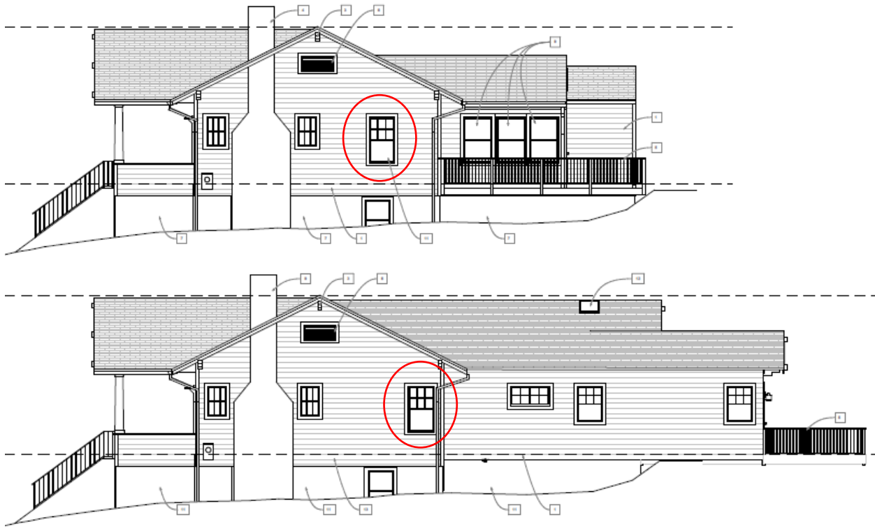
Figure 15: Existing north elevation (above) and proposed (below). On the main house, one existing original window will be relocated into a new opening to the right.
