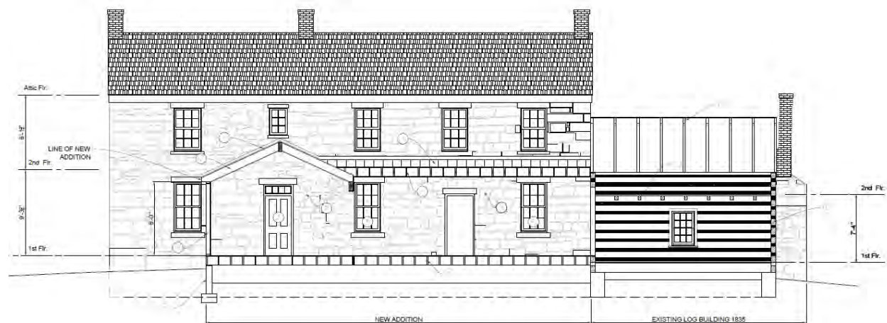
Figure8: Section cut through the addition showing the roof placement below the existing second-story window sills and retention of the historic rear wall and windows on the interior of the addition.
