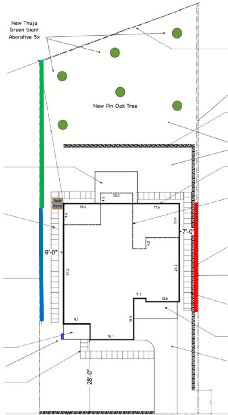
Figure 4: Staff's recommended fence condition recommends no fence be installed in the area shown in red; restricts the fence to no taller than 48" with an open picket design shown in blue and allows for a 6' privacy fence in the area shown in green.
