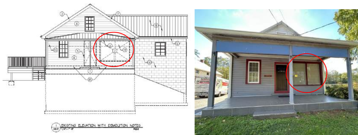
Figure 11: Front elevation showing the location of the picture window to be replaced.
