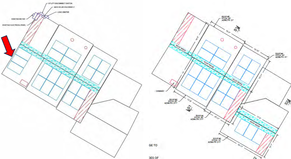
Figure 11: The proposed panel location for 7209 Willow Avenue (left) versus the approved panel location (right).
