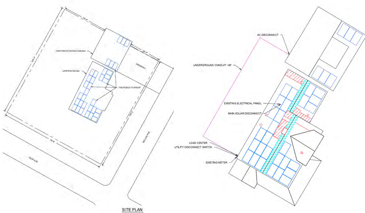
Figure 4: The site plan (left) shows the proposed solar panel locations and the building’s orientation toward Tulip and Willow Avenues. The roof plan (right) shows the proposed location of the solar panels and the equipment location.
