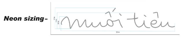
Figure 7: Detail of the neon lettering sizes.
