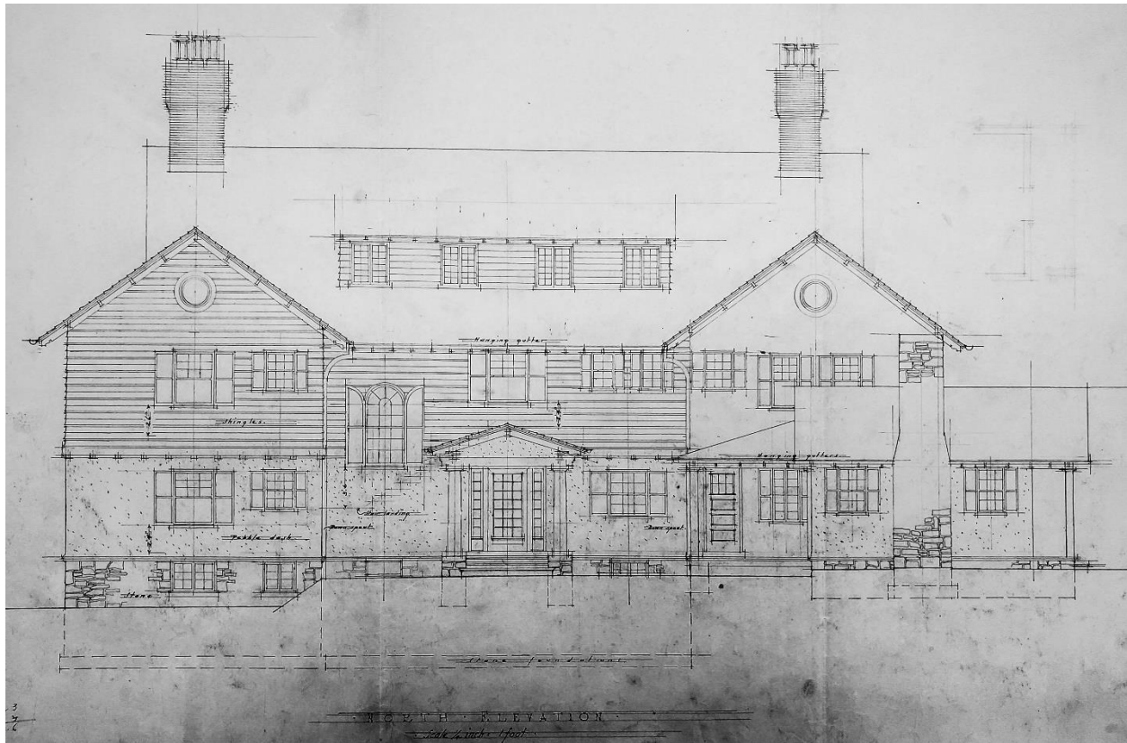
Figure 3: Drawings of north elevation, including front porch and semi-detached one-story kitchen structure on the northwest end, circa 1900. Source: Arthur B. Heaton Collection, Library of Congress, Prints and Photographs Division.
