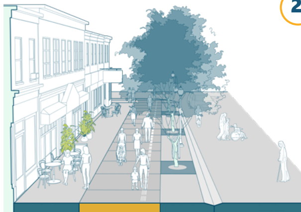
Figure 35. Diagram of a Shared Street with the Comfort Zone highlighted in yellow
