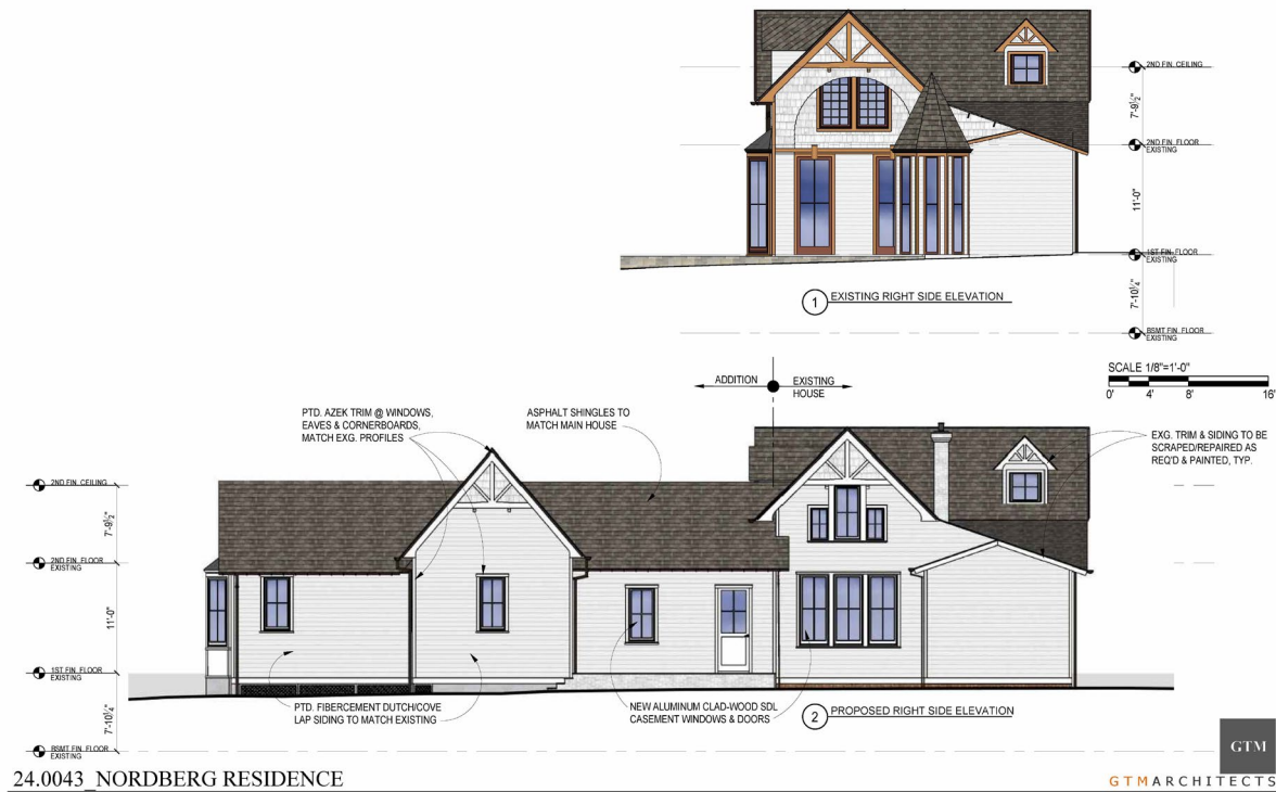
Figure 10: The existing right-side elevation, top, and proposed.
