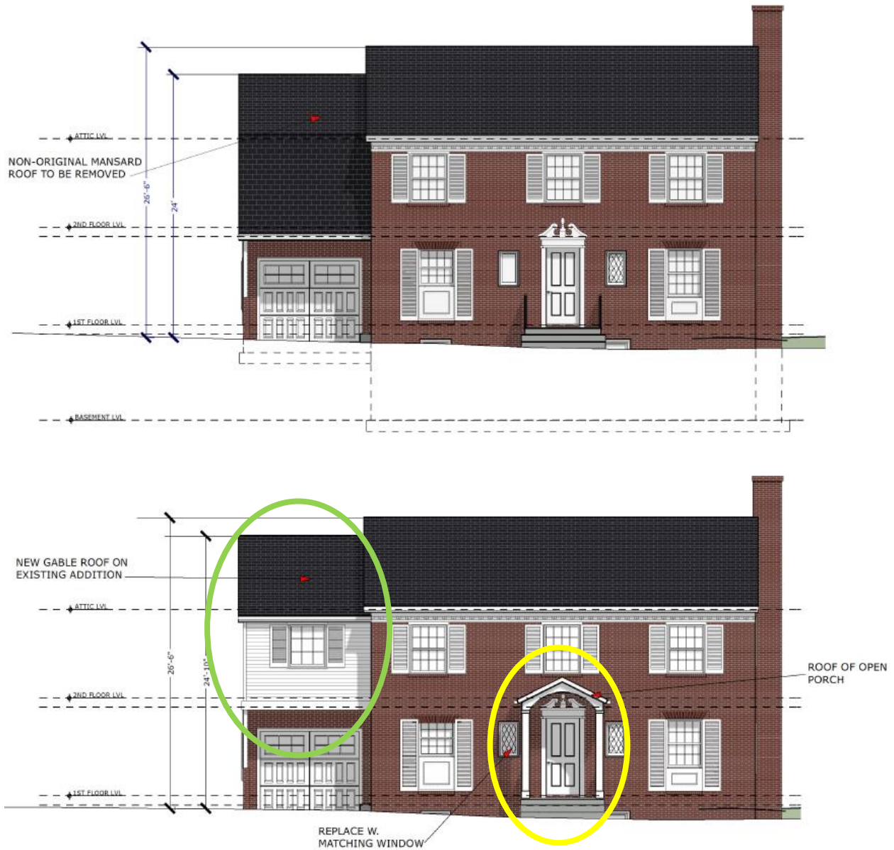
Figure 3: Proposed changes visible from the front including the front porch (circled in yellow) and the 2nd-story garage modification (circled in green).
