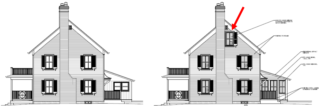
Figure 12: North elevation drawings, existing (left) and proposed (right). The red arrow points to the proposed casement window.
