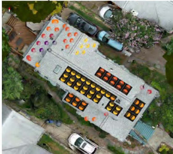
Figure 9: Shade map, left, and justification for panel location, right.
