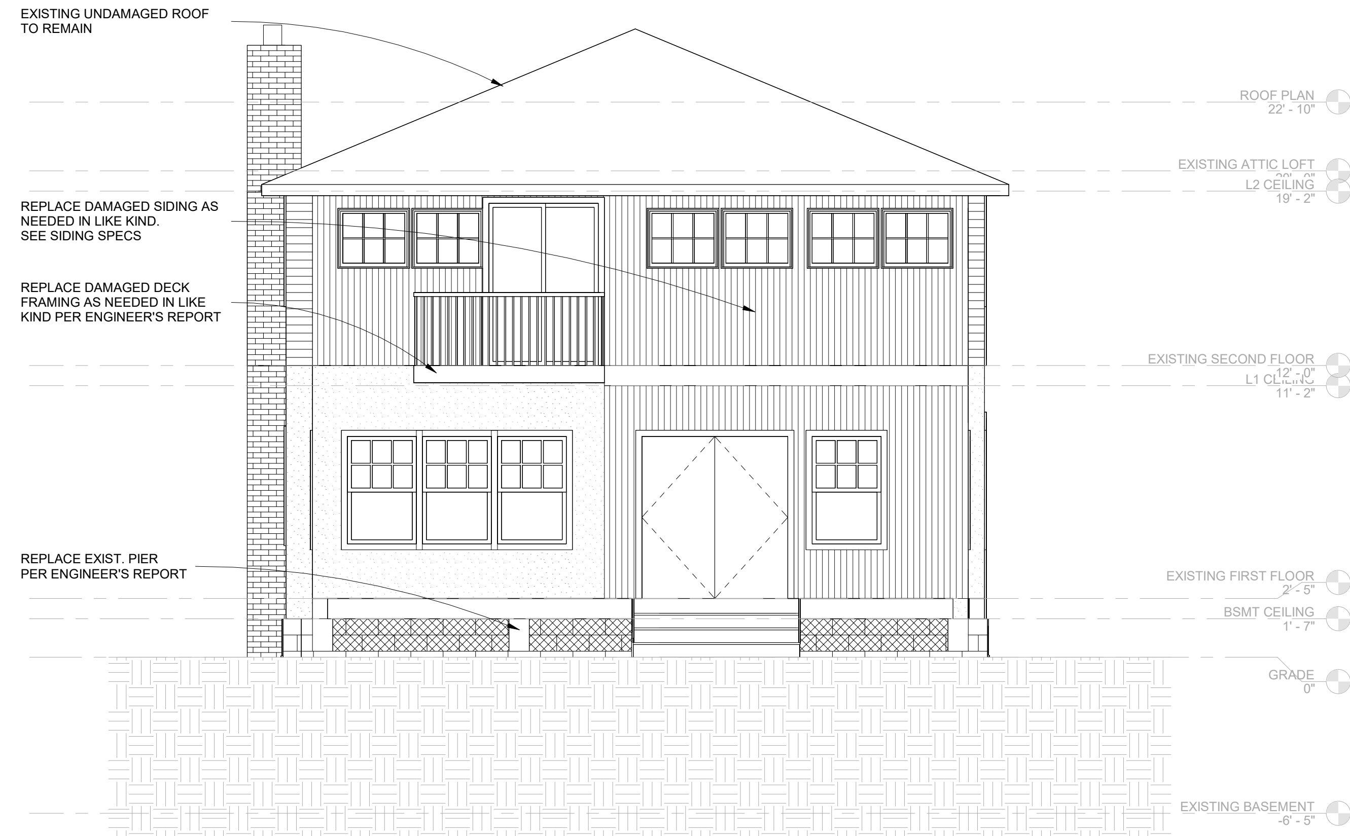
2 EXISTING REAR ELEVATION 1/4" = 1'-0"
