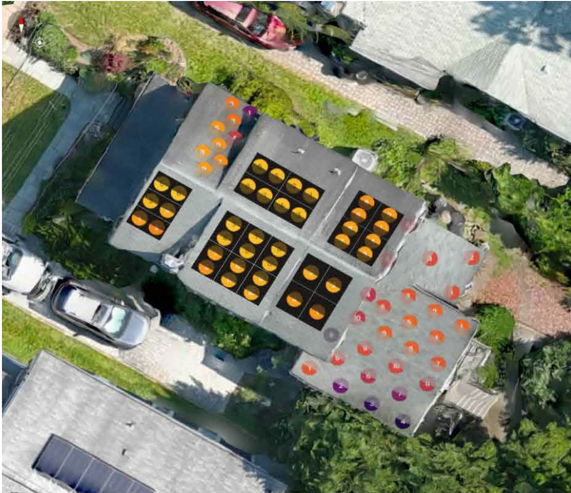
Figure 9: The shade map provided by the applicant shows the highest potential panel output in yellow. Orange indicates the middle point of production, and purple is the least productive.
