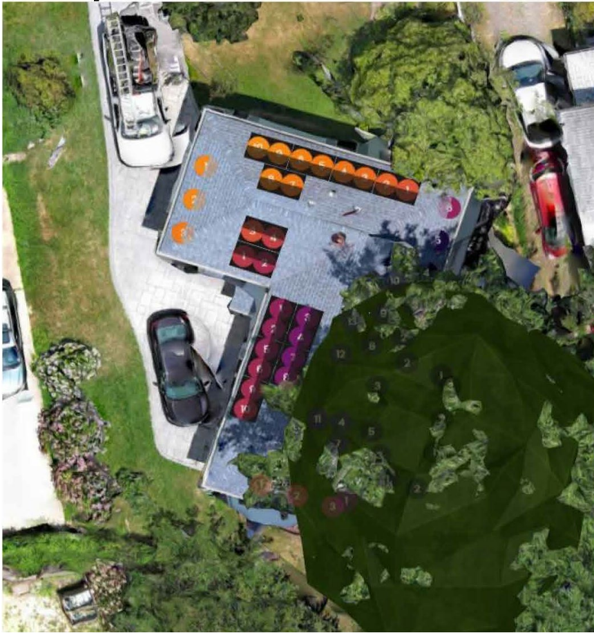
Figure 6: The shade map of the proposed panels provided by the applicant shows the most energy-productive roof planes in yellow and orange and the next most productive in purple.
