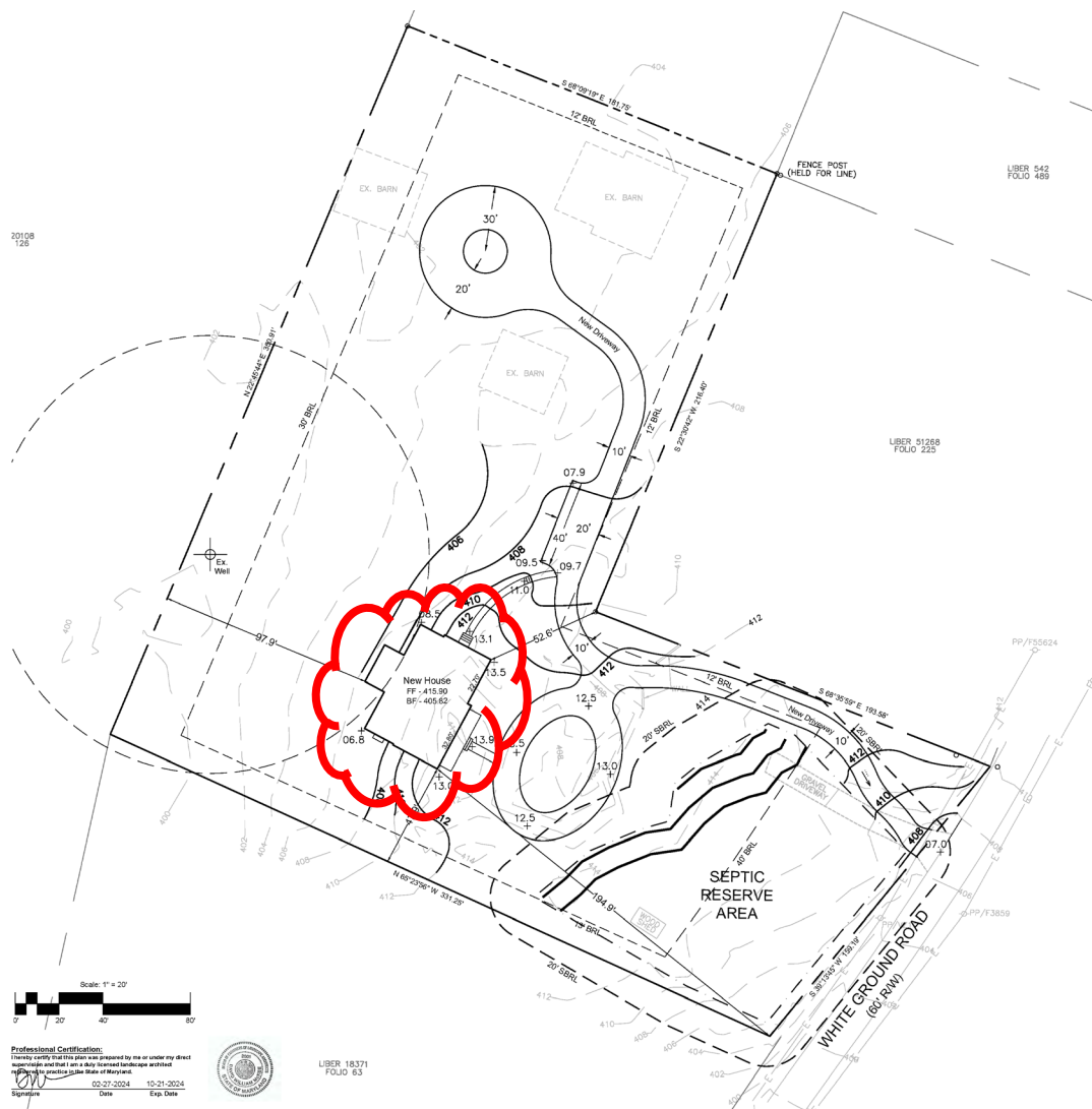
Figure 4: The proposed site plan for the subject property. The proposed building is clouded in red, 194.9 feet from the right of way.
