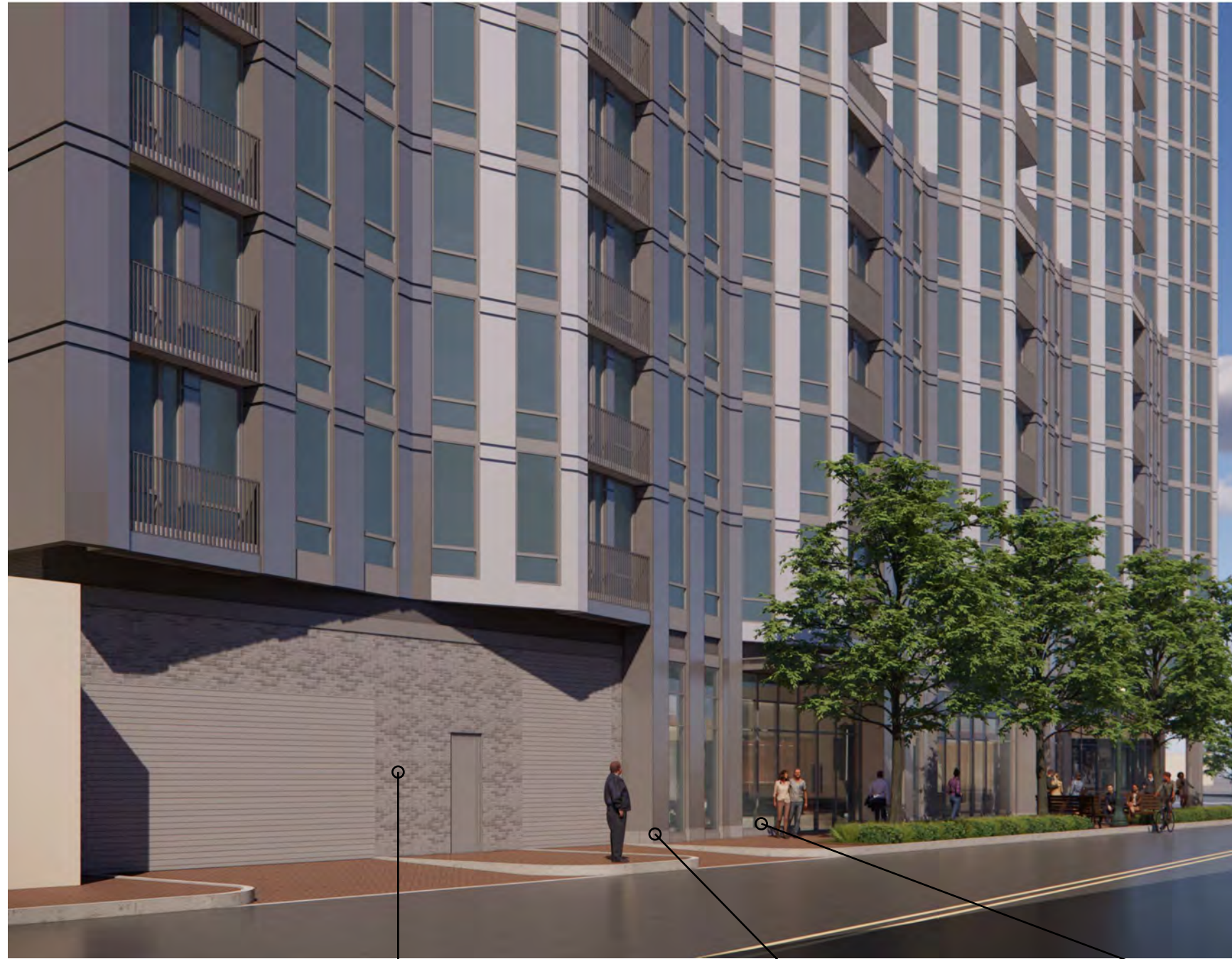
Masonry surround loading and garage entries
