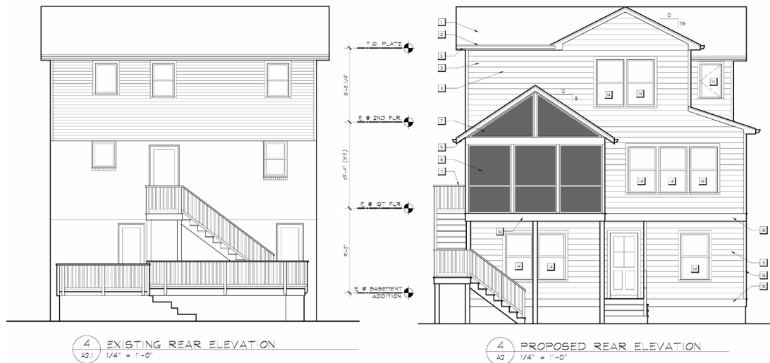
Figure 7: The existing, left, and proposed rear elevation.
