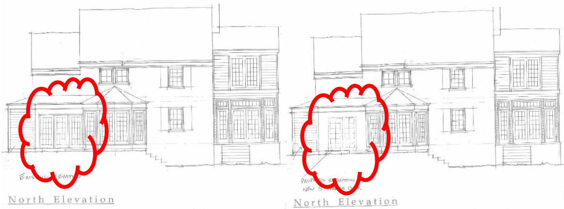
Figure 3: The existing, left, and proposed, right, north elevations with the existing and proposed doors clouded in red.
