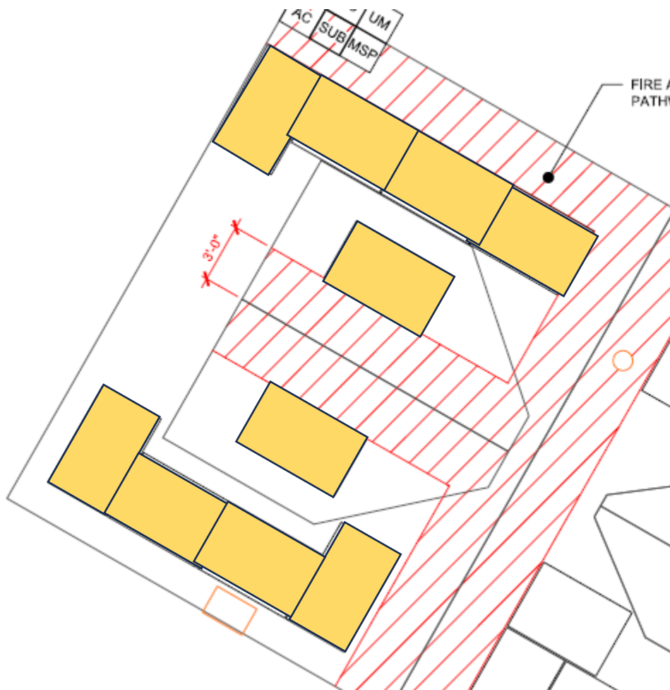
Figure 3: Detail of the propose solar panel arrangement on the street-facing roof side.
