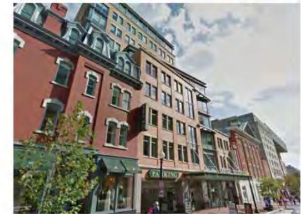
Building bases with variation in height and articulation can break up a large building, and can also reflect the modulation and character of adjacent structures. Source: Hariri Pontarini Architects (above), Google Street View (below)
